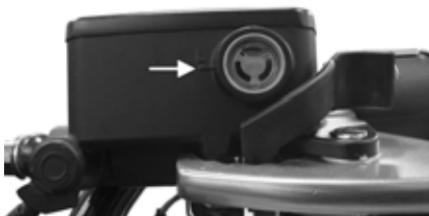
Check the brake fluid level in the auxiliary brake fluid reservoir.
