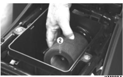
4. Place the element in a pan larger than the element and spray both sides generously with cleaning solvent. Let sit approximately three minutes.
