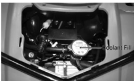
5. Install the radiator cap and access panel.
