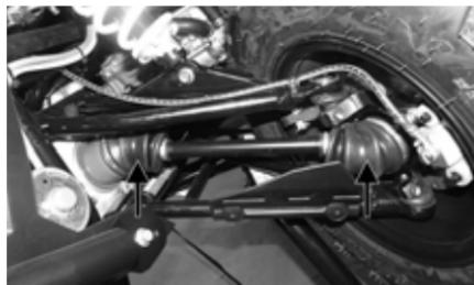
1. Inspect all drive axle boots for cracks, tears, or perforations.
