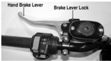
The hand brake is considered to be the normal operating (main) brake. It should be applied whenever a braking situation is needed.
