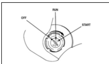
**OFF** position — All electrical circuits except the accessory are off. The engine will not start. The key can be removed in this position.
