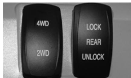
The left-hand 2WD/4WD switch allows the operator to operate the vehicle in either two-wheel drive (rear wheels) or four-wheel drive (all wheels). The right-hand switch allows the operator to mechanically lock the rear axle to apply equal power to both rear wheels. Both switches can be used together to achieve 4WD rear axle lock.
