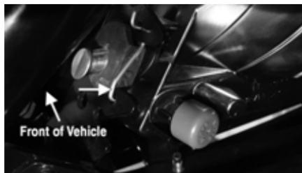
8. Install the wiring harness connectors
