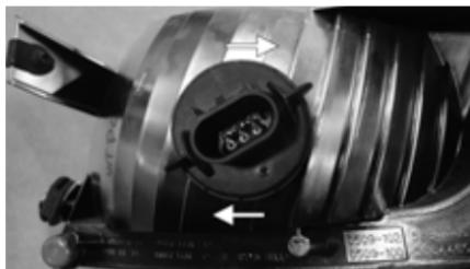
7. Headlight assembly mounts in a "C" shaped channel. Slide headlight assembly toward the front of vehicle to mount into "C" shaped channel. Install the retainers on both sides of the headlight assembly that secure the headlight assembly.
