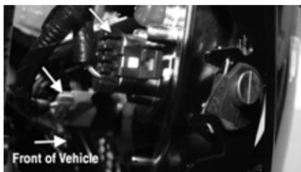
9. Install the headlight retaining knob.
