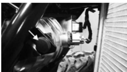
10. Adjust the headlight using the Checking/Adjusting Headlight Aim instructions in this section.
