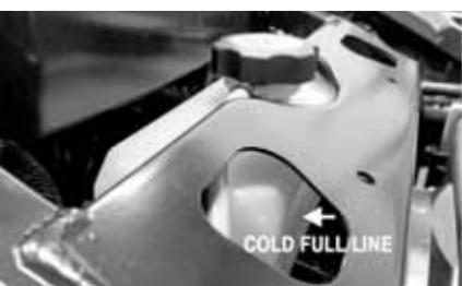
■ NOTE: If you cannot see any coolant in the reservoir, inspect the cooling system for leaks. If no leaks are present, add coolant using the bleed procedure below. If a coolant leak is suspected, schedule service with an authorized dealer.
