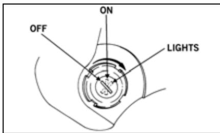
**OFF** position — All electrical circuits except the accessory plug are off. The engine will not start. The key can be removed in this position.
