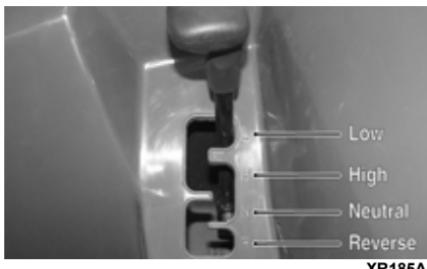
This ATV has a dual-range automatic transmission with reverse.
