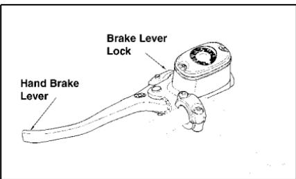
The hand brake is considered to be the normal operating (main) brake. It should be applied whenever a braking situation is needed.
