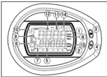
1. Speedometer/Tachometer/Condition Warning Display — Indicates the approximate vehicle speed (MPH or km/h) or RPM, and indicates a system error condition requiring attention.
