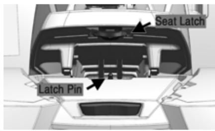
1. To remove the seat, lift up on the latch release (located at the rear of the seat); then raise the rear of the seat and slide it rearward.
