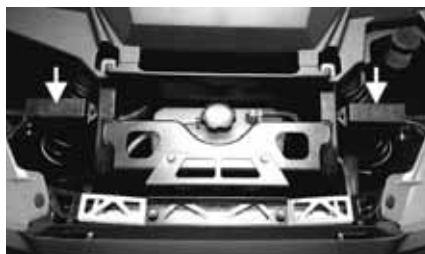
■ NOTE: To remove the fuse, compress the locking tabs on either side of the fuse cover and lift out.
