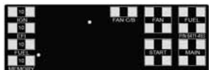
■ NOTE: To remove the fuse, compress the locking tabs on either side of the fuse cover and lift out.
